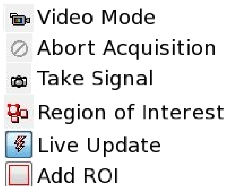
Fig. 3.— The most commonly used icons within the SOLIS software. These icons are useful when attempting to establish exposure times and other camera settings as they remove the need to trawl through drop-down menus.
